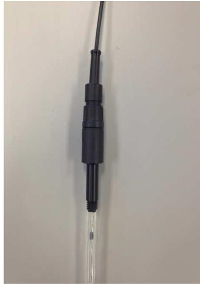
2. Connect the Y-cable to the electrode by screwing together the S7 connector of the Y-cable and the top of the electrode, as shown above. Hold the probe only by the plastic connector when doing this, not by the glass barrel.
