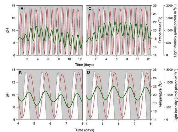
Sinusoidal temperature pH profiles. Smoothed (moving average) pH profiles of *N. oculata* when exposed to sinusoidal temperature. Two representative PBRs are shown (A & C, D). Top panels (A & C) display the entire experiment, while bottom panels (B, D) present in more detail the pH profile during the exponential growth phase (day 4 to day 8). White regions represent the sinusoidal light regime, thin red lines give the smoothed culture temperature and thick green lines show the pH profile.
